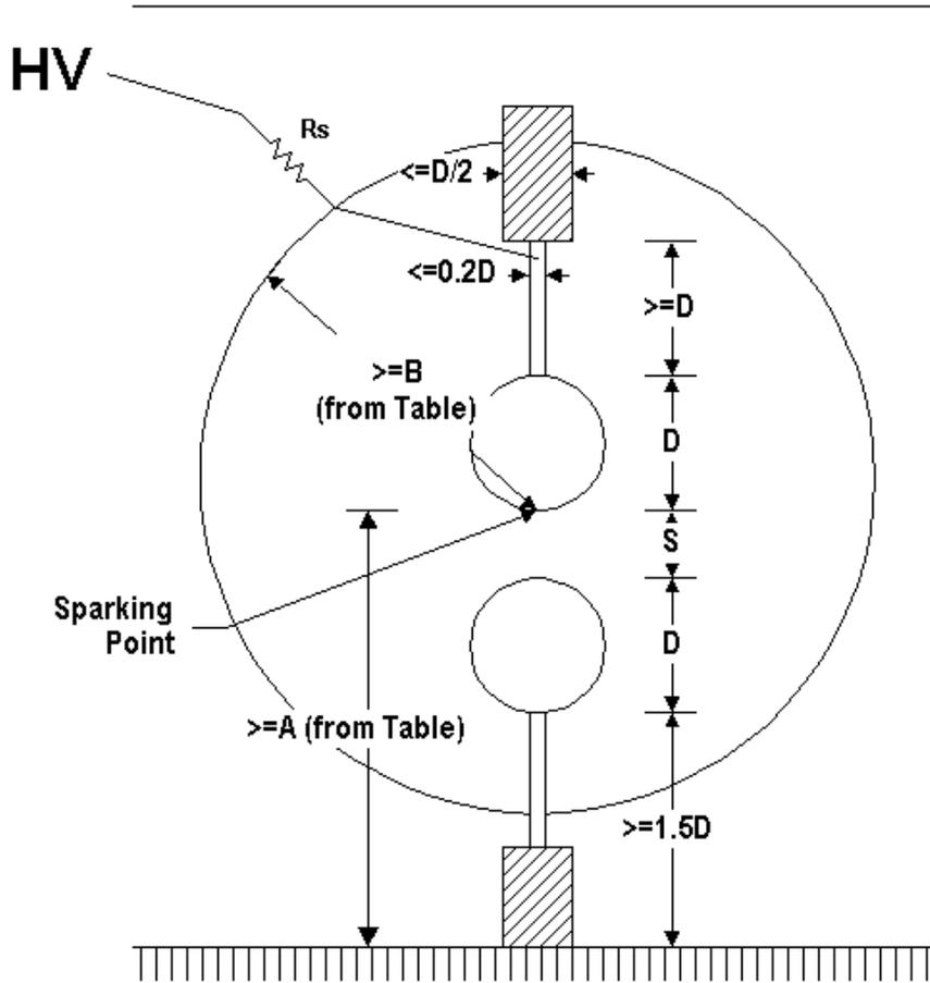
Horizontal gaps are much the same as vertical gaps, except that both electrodes are insulated. The insulators should be longer, at least  $2D$  long (putting the sparking point at least  $4D$  from the supports:  $2D$  for the insulator,  $1D$  for the shank,  $1D$  for the sphere). And, both spheres should be the appropriate clearance from the floor or external objects.
