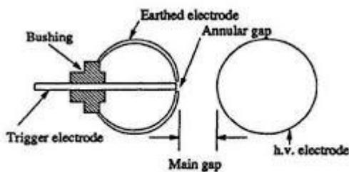
Figure:3.26 (a) Trigatron gap
