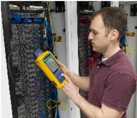
Cable test instruments are designed with a variety of focused features for particular field tasks. They vary in price, performance, and application. Depending on the task the field test instrument performs, it can be classified into one of the three hierarchical groups: certification, qualification, or verification. While some features overlap between test tools, each group answers a unique testing need and provides a different level of operational assurance.
